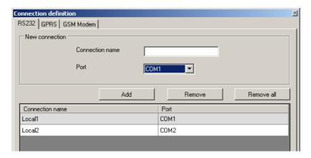
It is possible to do so with the above window that is available after activation of connection from Main Menu and selection Configuration tab or after clicking on icon on fast access bar and clicking on RS-232 tab.
