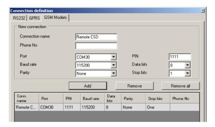
Click [Add] button to confirm settings and save connection (settings are inserted into table). Since that time a remote connection to device, reading and saving of parameters in PX100N memory is possible.
