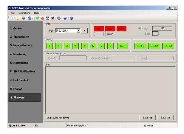
"Device Monitor" provides real-time information on device state. To use this function device must be connected to PC computer with LX-DATA cable (using DEBUG plug). Correct RS232 port must be chosen in "Port" field. "Device monitor" provides following information:
