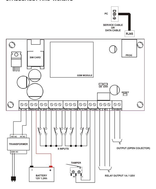
Connections of wires shall be made with due care to prevent any faults or dead shorts. Places of connections shall be protected against weather conditions. According to the above figure terminals of transmitter shall be connected to:
