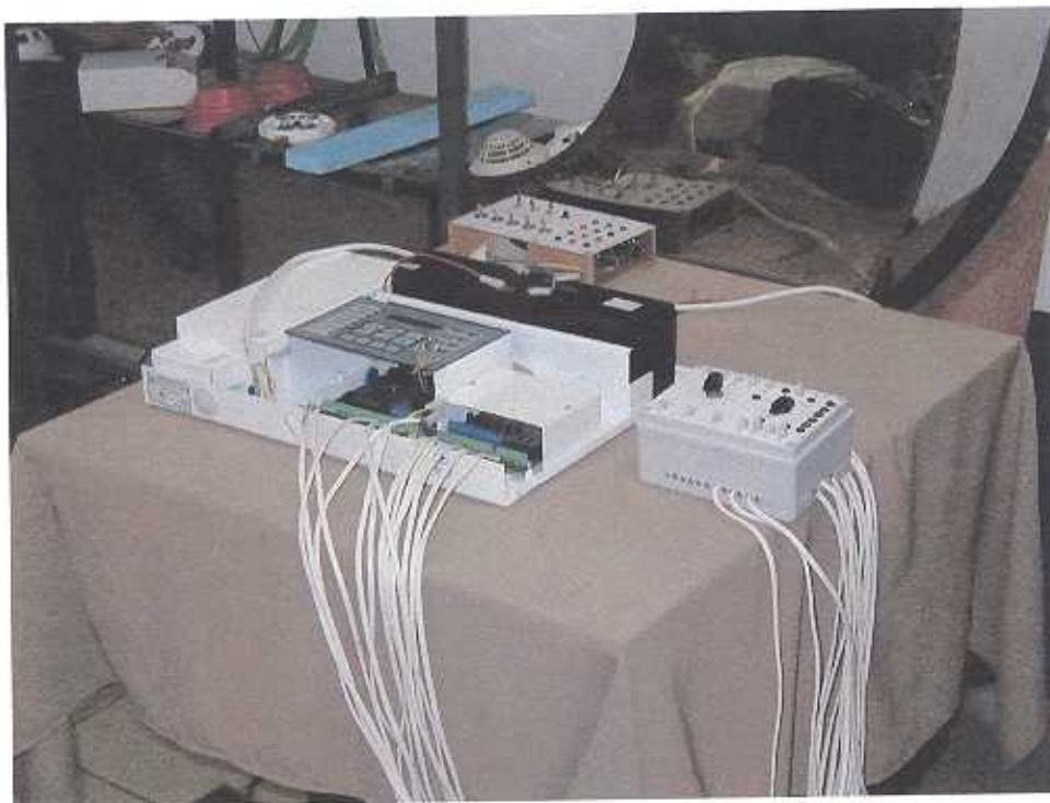
Photo 2: Fire Control Panel FS 5100 with Technical Appliances
