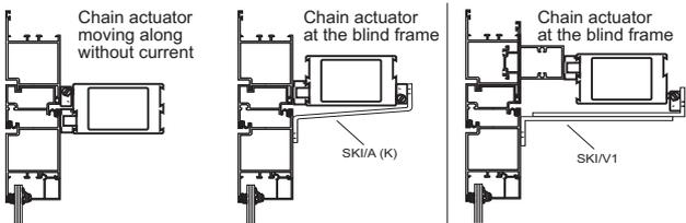
Wing excess end 0 - 12 mm (when the excess end is 13 - 22 mm, please apply distance guide blocks)
