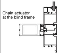
Wing excess end 0 - 12 mm (when the excess end is 13 - 22 mm, please apply distance guide blocks)
